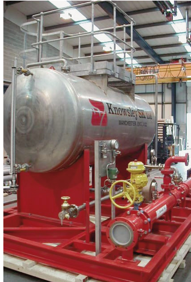
Figure 1. Typical 3P foam skid with actuated control valve
