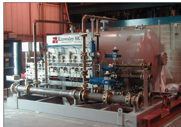
Figure 4. Bladder tank construction at the KSK workshop
